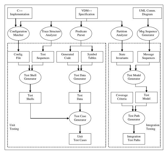
Figure 5.1. Architecture of the SpecTGS
