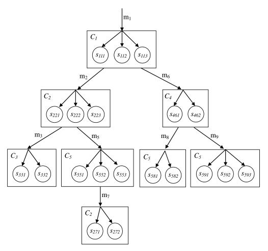
Figure 6.9. A test model for the message sequence (*m1* (*m2* (*m3*) (*m5* (*m7*))) (*m6* (*m8*) (*m9*)))
