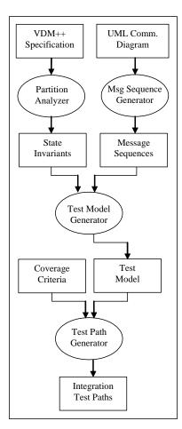
Figure 6.1. Integration testing part of the SpecTGS framework
