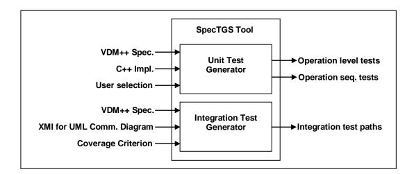
Figure 7.1. Architecture of the SpecTGS Tool
