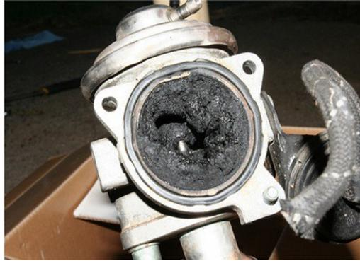
FIGURE 1.3: Chocked EGR actuator [3]
