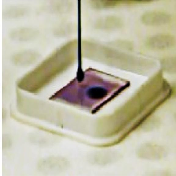
FIGURE 3.3: Drop casting process for the growth of organic thin films.
