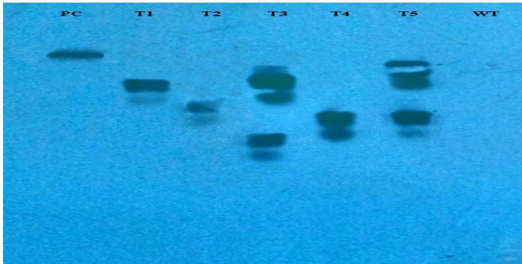
FIGURE 4.14: Southern blot analysis of PCR-positive plants demonstrating the incorporation of *rol A* gene into the *Artemisia carvifolia* genome. T1-T5 represents *rol A* transgenics. “PC” indicates plasmid DNA as positive control. “WT” represents wild type plants with no *rol A* gene. Transgenic lines T3 and T4 showed two copies of integrated gene.
