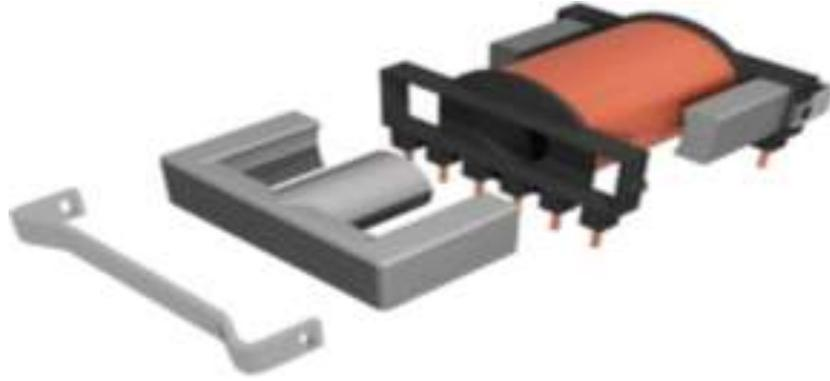
FIGURE 3.28: Ferrite core transformer in E-core shape [149].
