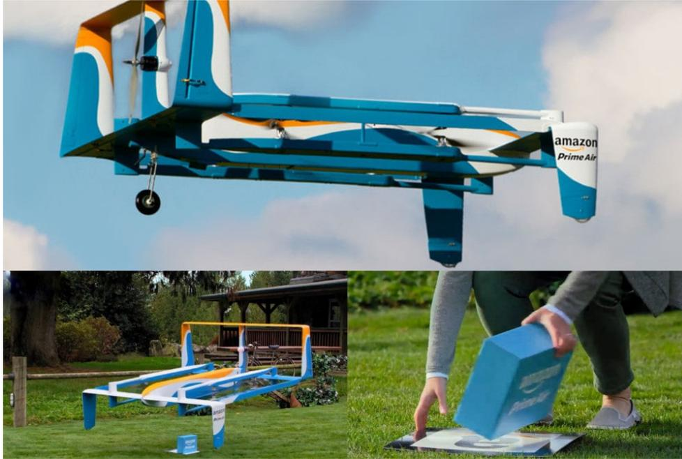
FIGURE 1.5: Unique Fixed-wing Hybrid VTOL UAV used by Amazon Prime Air
