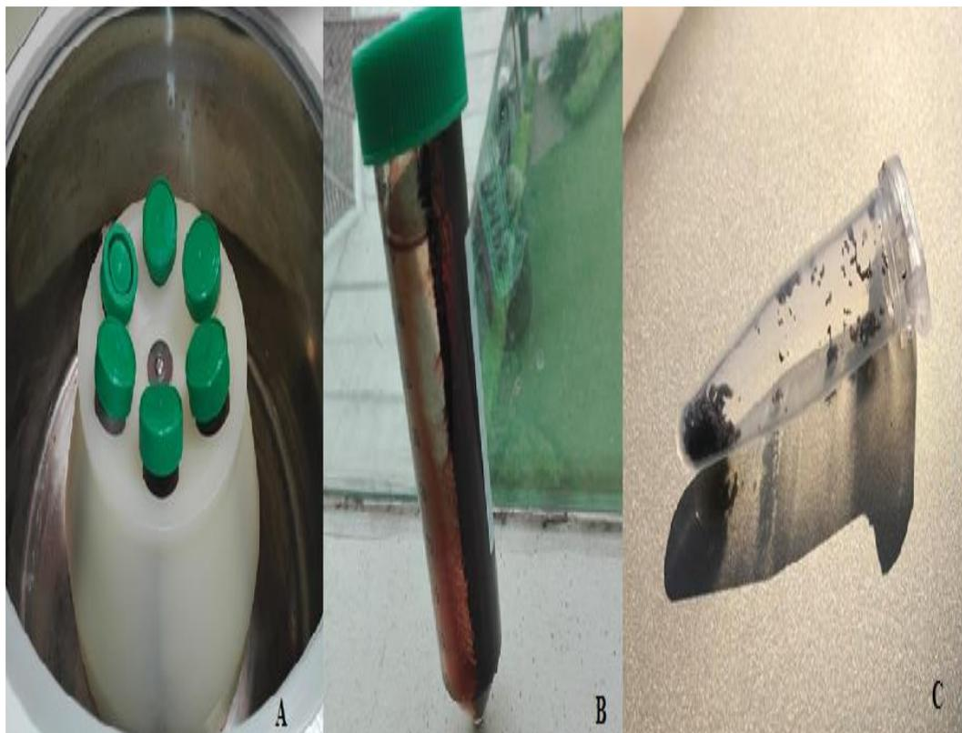
FIGURE 4.2: Silver nanoparticles after centrifugation (A and B). Synthesized silver nanoparticles in powder form (C).
